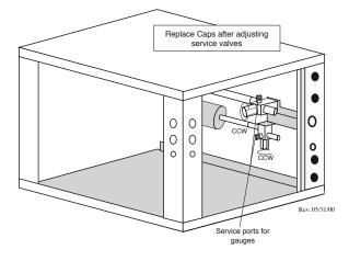
Figure 5: Service Valve Positions
